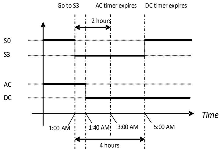
**Figure 9-52 System transitions with WakeAlarm -- Timer**
