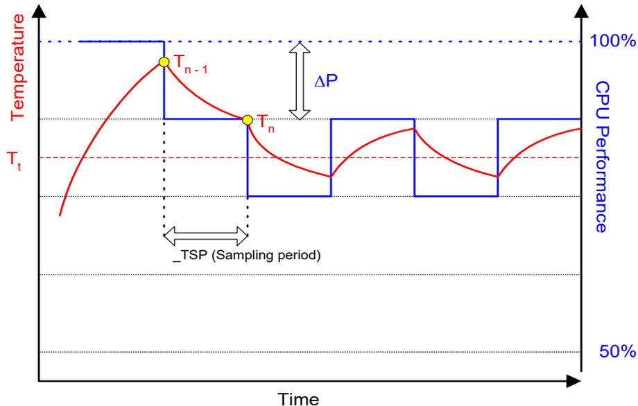
Figure 11-63 Temperature and CPU Performance Versus Time
