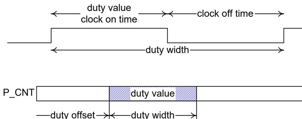
**Figure 8-37 Throttling Example**
