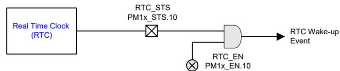
**Figure 4-11 RTC Alarm**
