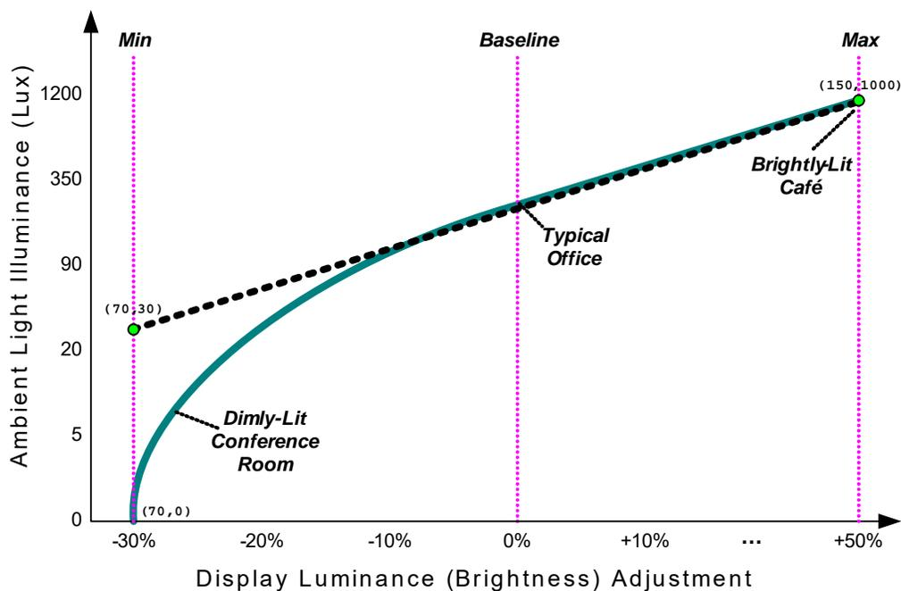
**Figure 9-48 A two-point ALS Response Curve**
