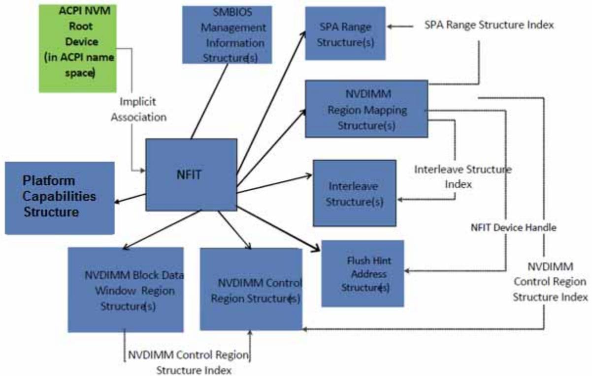
Figure 5-22 NVDIMM Firmware Interface Table (NFIT) Overview
