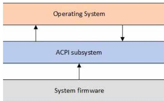
The *ACPI subsystem* is an interface layer between the *System firmware* and the *OS*. The arrows indicate data flow.
