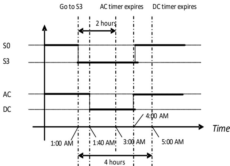
**Figure 9-53 System transitions with WakeAlarm -- Policy**
