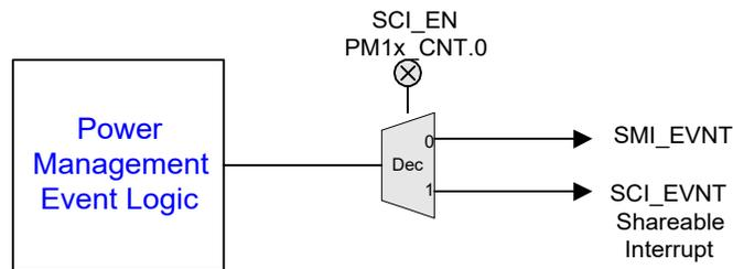
**Figure 4-12 Power Management Events to SMI/SCI Control Logic**
