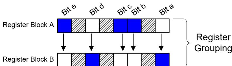
**Figure 4-5 Example Fixed Hardware Feature Register Grouping**
