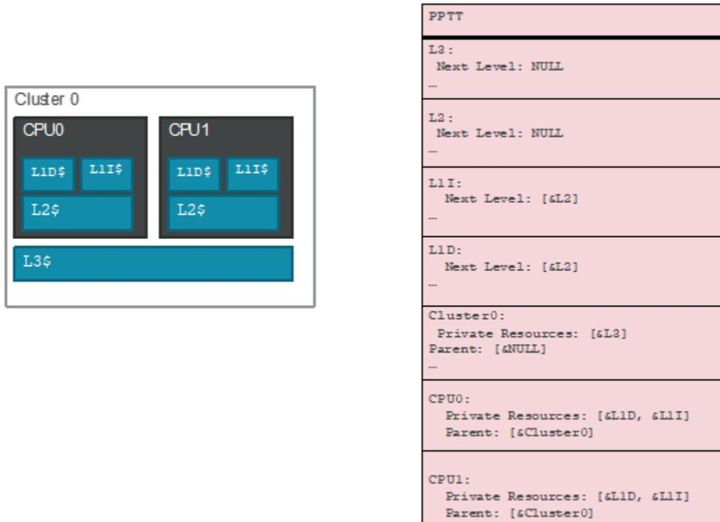
**Figure 5-26 Cache Type Structure - Type 1 Example**
