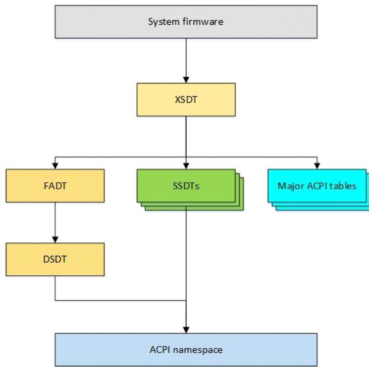
*System firmware* updates the ACPI tables as necessary with information only available at runtime before handing off control to the bootstrap loader.
