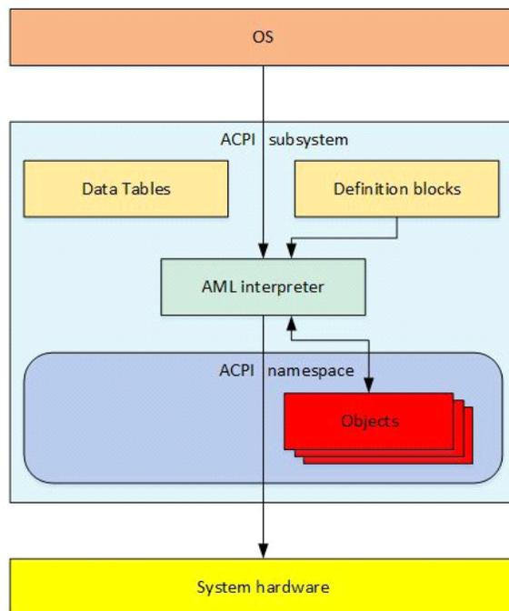
The ACPI subsystem consists of two types of data structures: *data tables* and *definition blocks*.
