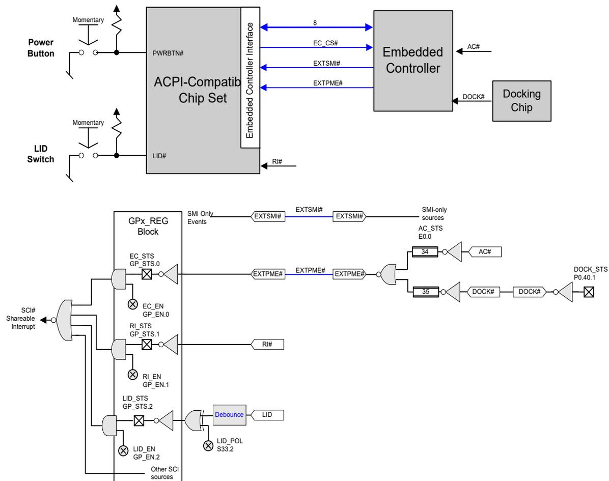
**Figure 4-13 Example of General-Purpose vs. Generic Hardware Events**
