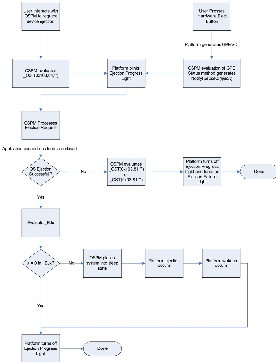
Figure 6-34 Device Ejection Flow Example Using \_OST
