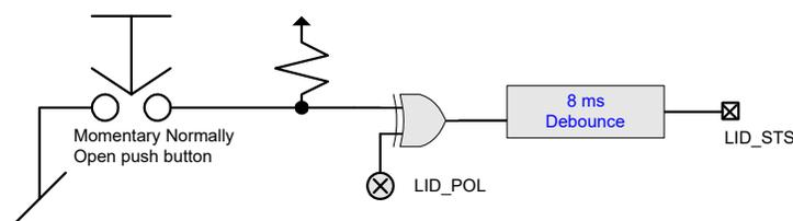
**Figure 4-14 Example Generic Address Space Lid Switch Logic**
