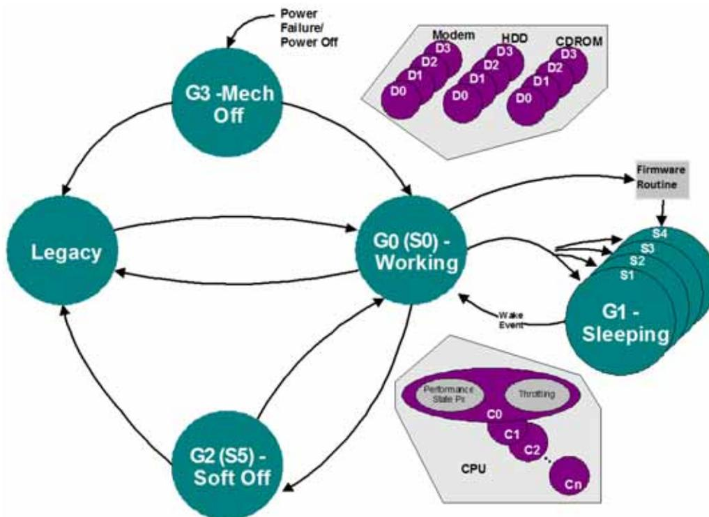
**Figure 3-1 Global System Power States and Transitions**
