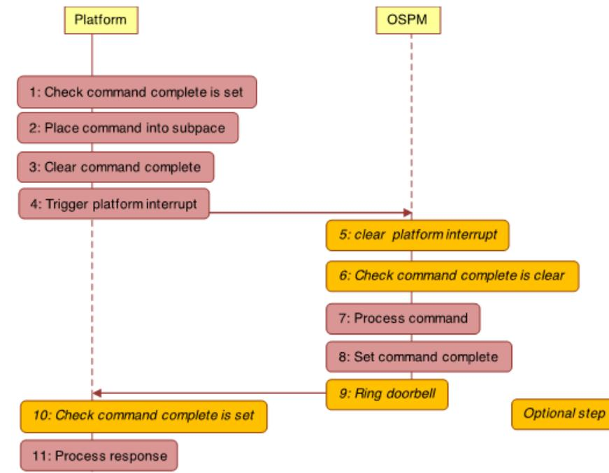
**Figure 14-73 Communication flow for notifications on slave subspaces**
