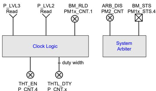
Figure 8-40 ACPI Clock Logic (One per Processor)
