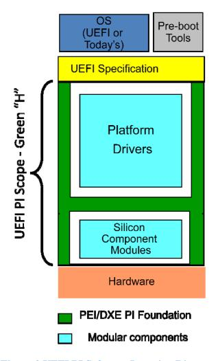
Figure 3 UEFI PI Software Layering Diagram
